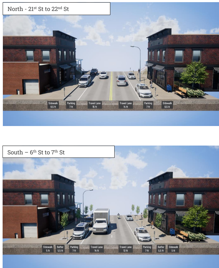
Figure 7: Central Avenue Typical Roadway Sections
