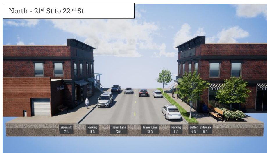
Figure 8: White Street Typical Roadway Sections
